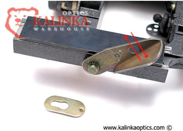
Step 6: Simply slide the clip back into the indentation. Try the fit, make sure the scope will slide onto the plate easily, and will also tighten up. There should be a moderate amount of tension on the lever when it is about 85 percent closed, and it should take mild pressure to lock it completely. Do not over-tighten. Repeat the procedure to adjust the tension if needed.
